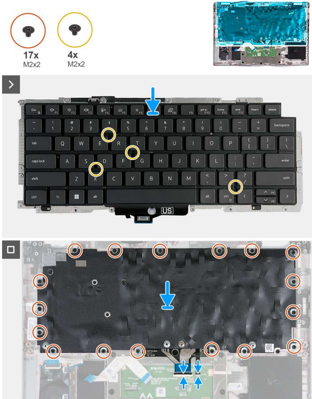
Figure 62. Installing the keyboard
