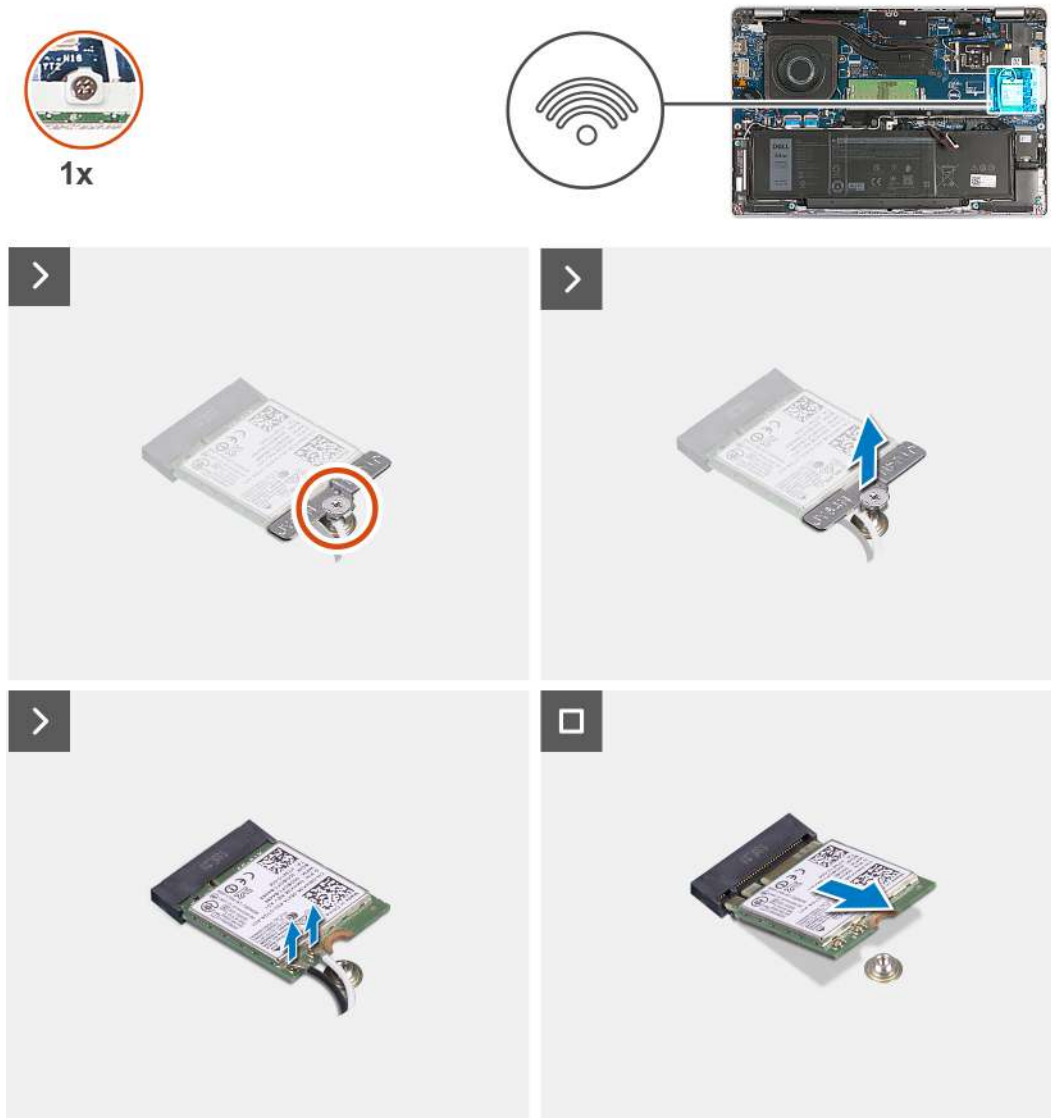
Figure 10. Removing the wireless card
