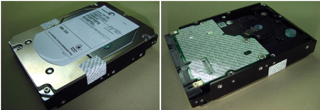
Figure 7. Example of FIPS tamper evidence labels.
